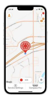
Through the App, the response team has access to information about what the device has detected (e.g., arc flash, fall, or impact), as well as geo-location information and the user's responses, if any. Set up much like a text thread, notifications are recorded and time stamped in a "chat" that enables the user to communicate with the response team when able.
