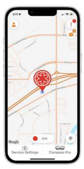
Through the app, the response team has access to information about what the device has detected (e.g., arc flash, fall, or impact), as well as geo-location information and the user's responses, if any. Set up much like a text thread, notifications are recorded and time stamped in a "chat" that enables the user to communicate with the response team when able.
