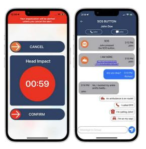
Anytime an alert is triggered by detecting an adverse event, the device will begin a 60-second countdown, during which the user can cancel the alert. After that period, the App will notify the designated response team, which is determined by the contacts input during App set-up. The notification will indicate the basis for the alarm; for example, that the unit has detected an arc flash or an impact. The
