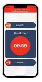
The purpose of the timer is to allow the user a limited window of time in which to disable the alert, in the case of a false alarm or in cases where the worker may have suffered an event, but does not need medical assistance.
